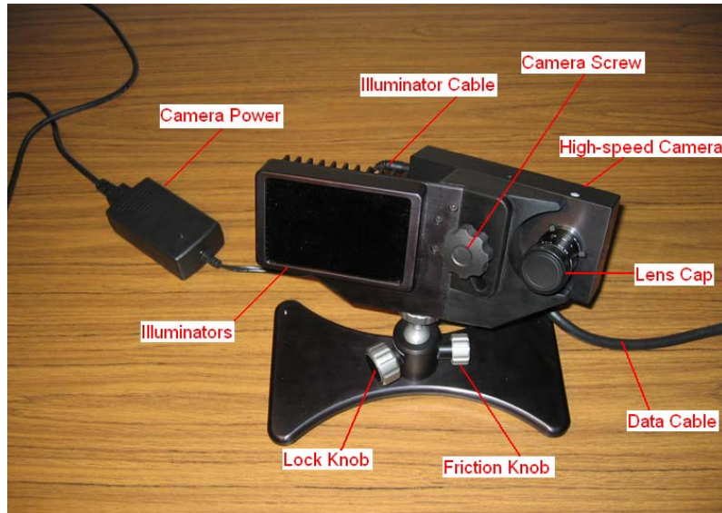
Figure 4-1: EyeLink 1000 Desktop Mount Components
