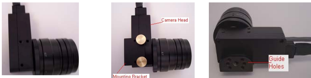
Figure 7-3: Fiber Optic Camera Head with lens (left), attached to the Bracket (center), Guide Holes in the Bracket accept Guide Pins from Camera Head Clip (right)
