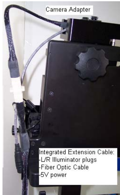
Figure 3-7: Fiber Optic Camera in the Tower Mount
