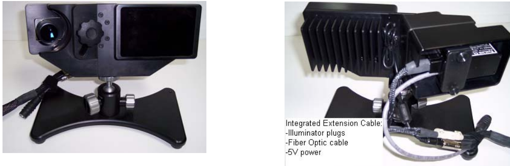
Figure 4-6: Fiber Optic Camera in the Desktop Mount viewed from the front (left) and rear (right)
