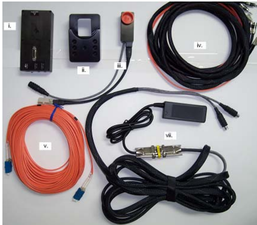
Figure 2-3: Fiber Optic Camera Components.
