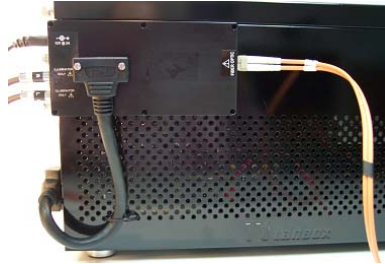
Figure 2-4: Camera Base Box and Cabling affixed to the side of the Host PC
