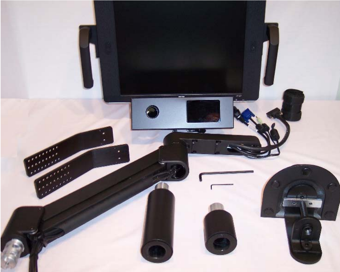
Figure 5-2: EyeLink 1000 LCD Arm Mount Components: LCD Arm Mount Base, Arm, Camera and LCD Assembly
