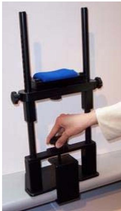
Figure 3-2: Clamping Chinrest to Table
