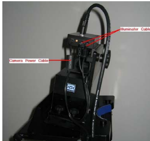
Figure 3-6: Camera and Illuminator Cables for a Standard Camera Used in the Tower Mount
