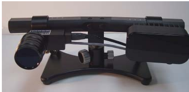
Figure 1-6: Typical EyeLink 1000 Long Range Mount Configuration
