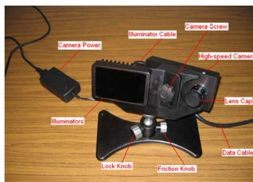
Figure 3-5: Parts of the EyeLink 1000 Desktop Mount
